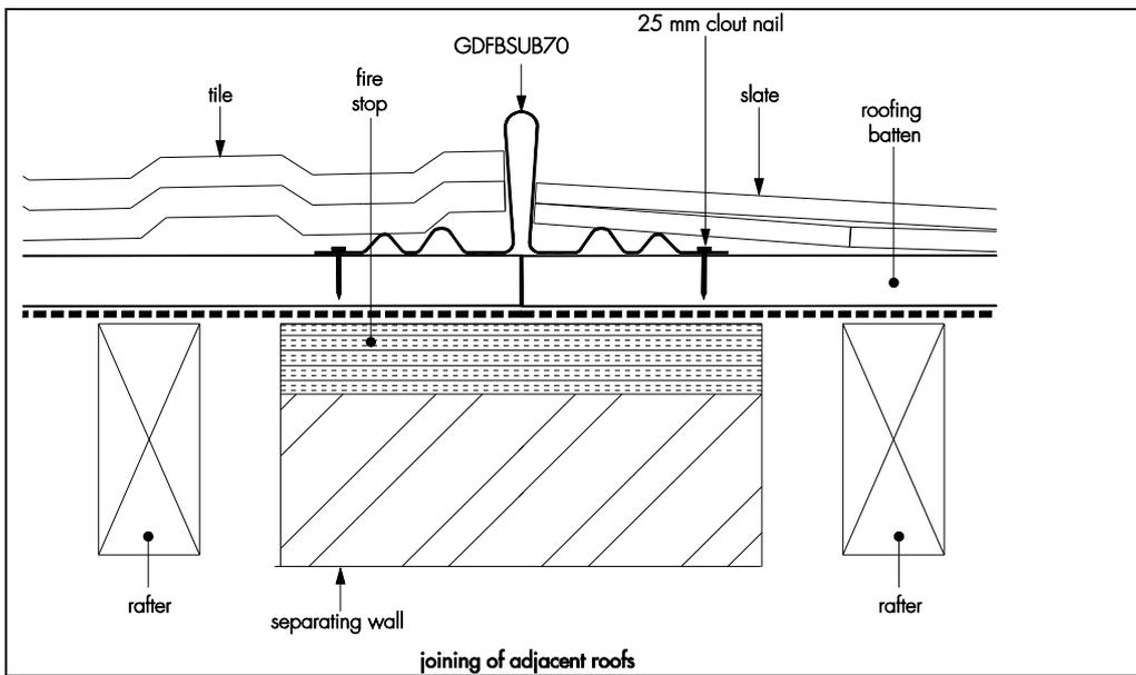
Figure 4 Filon GRP Dry Fix Bonding Strip – GDFBSUB 100
