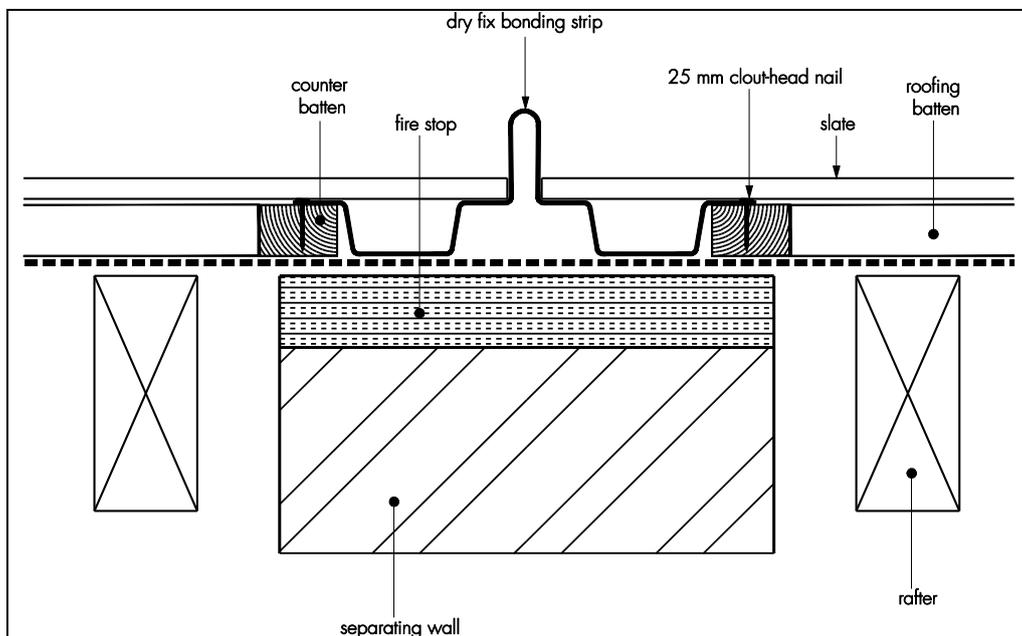
Figure 2 Filon GRP Dry Fix Bonding Strip – GDFBS 110
