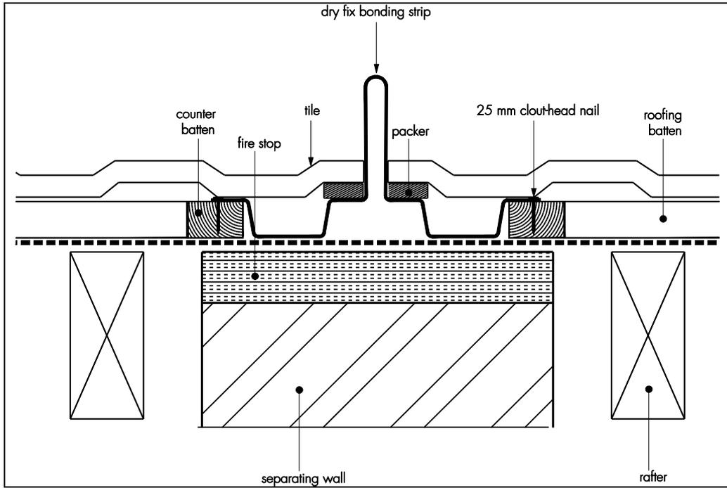
Figure 3 Filon GRP Dry Fix Bonding Strip – GDFBSUB 70
