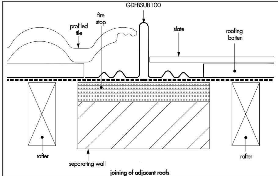
1.2 The profiles are supplied in lengths of 3 m, with widths of 225 mm and depths of 70 mm (GDFBS 70 and GDFBSUB 70), 100mm (GDFBSUB 100) and 110 mm (GDFBS 110).
