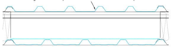
Over-roof rooflight sheet types to achieve Class B non-fragility in a Class B non-fragile roof (see also TIS101)
