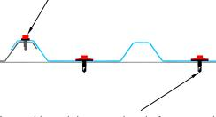
Austenitic stainless steel main fasteners that incorporate minimum 29mm diameter sealing washers @ maximum 200mm centres. Minimum 19mm diameter sealing washers may be used with a CE36E, CEDR30E or Supasafe E sheet subject to wind loads
