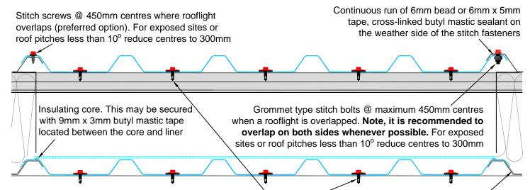
Minimum 5.5mm diameter austenitic stainless steel main fasteners that incorporate minimum 29mm diameter sealing washers @ maximum 200mm centres for outer sheets or minimum 5 fasteners per sheet width for liners. Minimum 19mm diameter sealing washers may be used with a CE36E, CEDR30E or Supasafe E sheet subject to wind loads.
