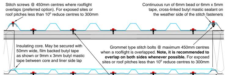
Minimum 5.5mm diameter austenitic stainless steel main fasteners that incorporate minimum 29mm diameter sealing washers @ maximum 200mm centres for outer sheets or minimum 5 fasteners per sheet width for liners. Minimum 19mm diameter sealing washers may be used with a CE36E, CEDR30E or Supasafe E sheet subject to wind loads.
